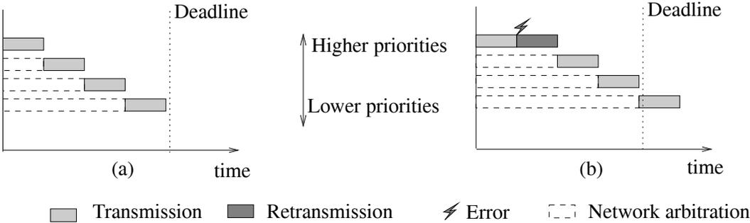
**Figure 1. Message transmission over a priority-based network.**
